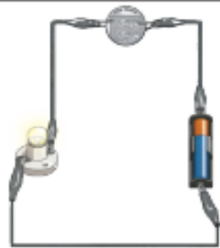
10p = metal = electrical conductors
